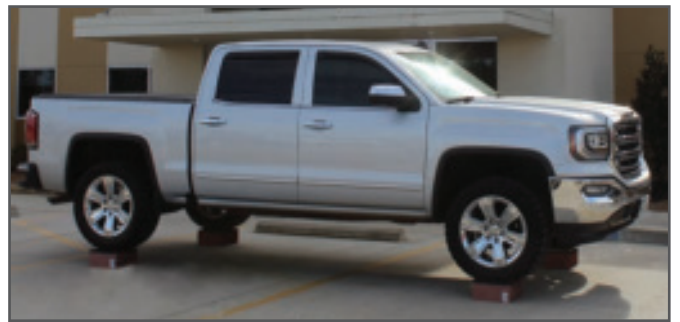
We took four pieces of our standard 6" thick Kuul Control evaporative media and let them fully support the weight of a 4000+ pound truck. The media suffered little to no damage.
