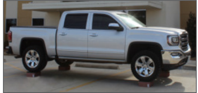
We took four pieces of our standard 6" thick Kuul evaporative media and let them fully support the weight of a 4000+ pound truck. The media suffered little to no damage.
