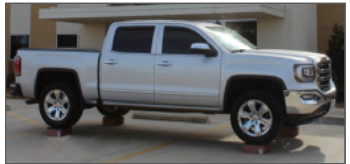
We took four pieces of our standard 6" thick Kuul Vitality media with DuraPro and let them fully support the weight of a 4000+ pound truck. The media suffered little to no damage.
